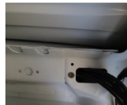
Excess rear switch harness to be tucked in cavity in pillar above rear switch
