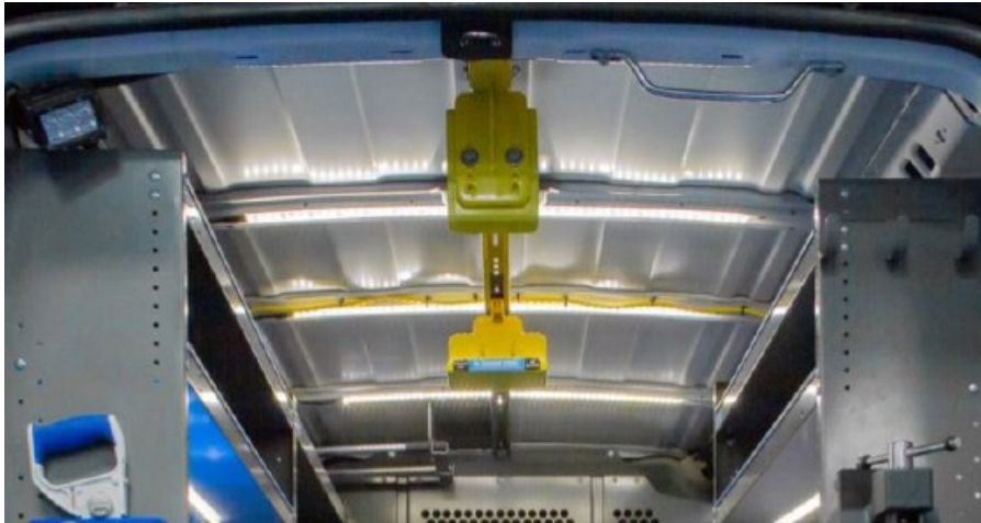
36" LED Light Strip Installed
