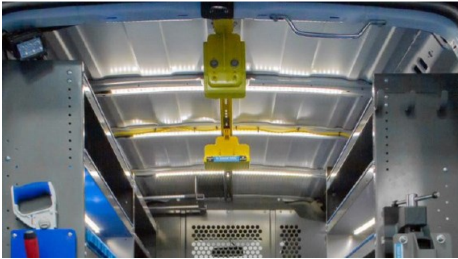
LED Light Strips Installed
