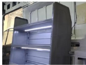
Install from Transit. The P-HARRB3 will come down on the left side of bin vs right in picture
