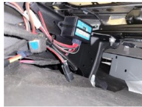
VTM mounted to underneath and back of driver seat bracket and VTM harness wire tied to bracket
