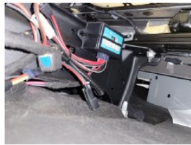
VTM mounted to underneath and back of driver seat bracket and VTM harness wire tied to bracket
