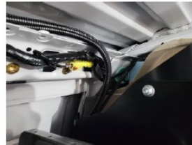
VTM harness routed up street side B pillar
