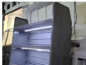
Install from Transit. The P-HARRB3 will come down on the left side of bin vs right in picture
