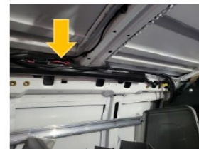
CL-ADP to be added onto Vehicle Specific Harness
