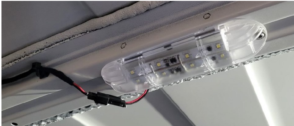
LED Dome Light Installed on Roof Bow
