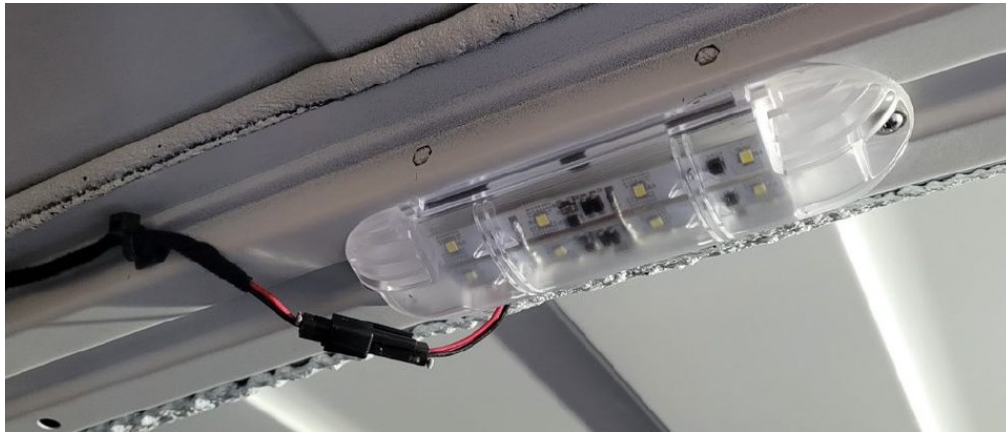
LED Dome Light Installed on Roof Bow
