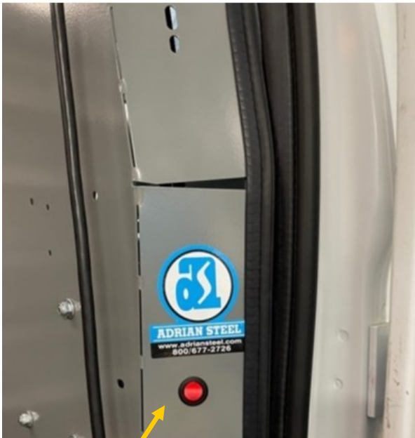
Steel partition hole behind passenger seat
