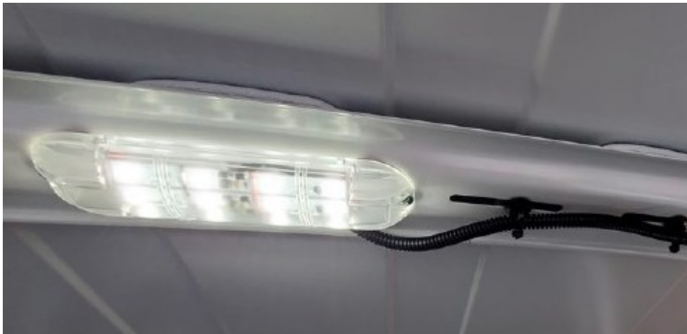
LED Dome Light Installed on Roof Bow
