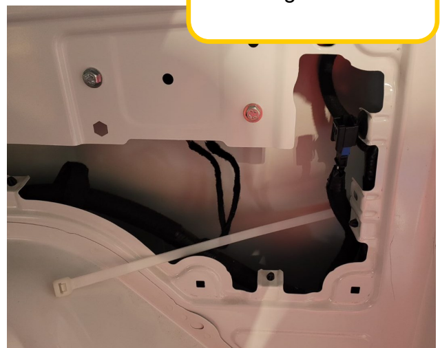
Remove panel to drill the hole and to route the wiring
