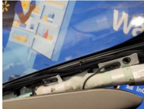
VTM harness cable tied to factory harness in passenger A pillar
