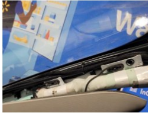
VTM harness cable tied to factory harness in passenger A pillar
