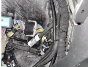
Harness ran up the passenger kick panel and into the A pillar
