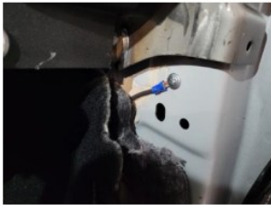
Ground for timer module
