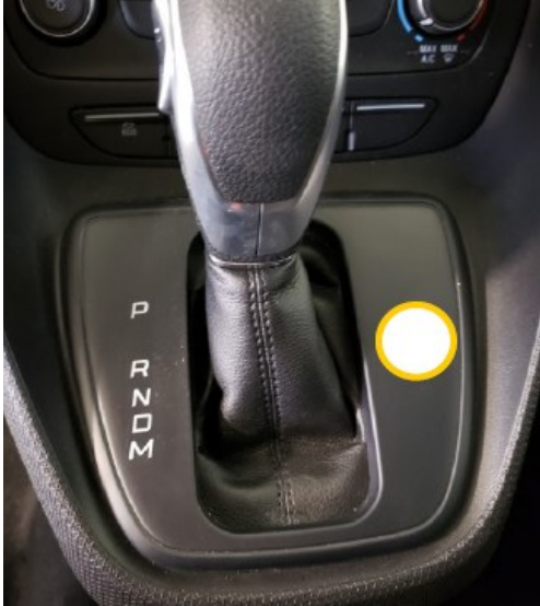
Switch placement: On Shift Column Panel
