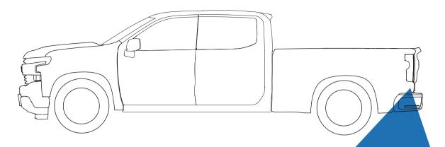
OEM tail lamp connection and backup alarm placement are below driver side tail lamp
