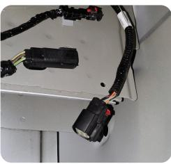
**STEP 3:**Install the P-BUA-COLORADO harness between the two OEM connectors
