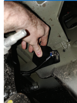
Backup alarm is located on the street side of the driver side frame rail; below the driver side tail lamp cavity
