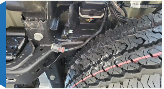
OEM tail lamp connector is inside driver side frame rail above spare tire
