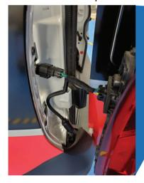
Backup alarm is located on street side of driver side frame rail, directly below driver side tail lamp
