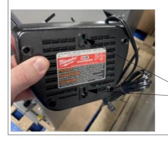
TIGHTEN NUT ON SCREW TO SET DISTANCE UNTIL CHARGER SLIDES SNUG OVER SCREW HEADS.
