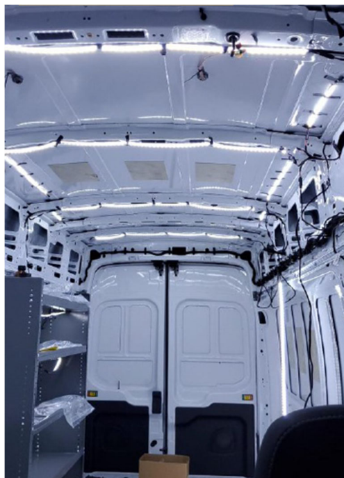
LED Light Strips Installed
