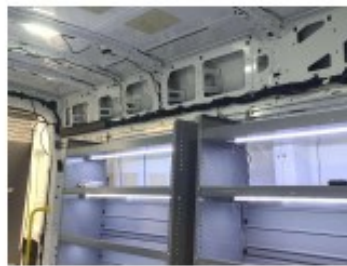
CL-48BLED lights added to rear street side cargo racks on 3 of the top shelves, and CL-36BLED added to front 3 of the top shelves
