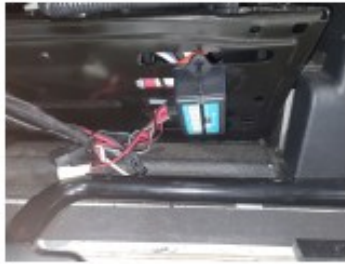
Module to be placed under and behind driver seat on back of seat mount.
