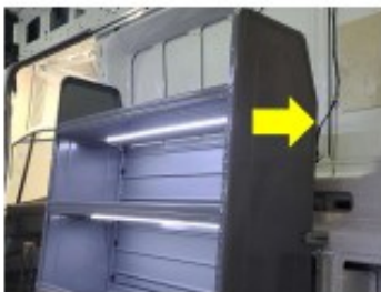
CL-36BLED lights added to top and middle shelves of cargo rack. Note P-HARRB4 ends and P-HARRB1 is added for an extension
