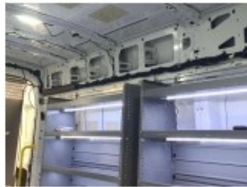
CL-48BLED lights added to rear street side cargo racks on 3 of the top shelves, and CL-36BLED added to front 3 of the top shelves
