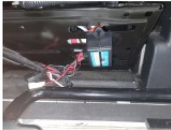
Module to be placed under and behind driver seat on back of seat mount.
