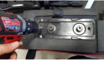
Make a mark 1.5" toward the outside of each mounting bolt and drill holes with a 3/8" drill bit.
