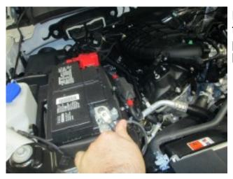
Remove OEM battery cable from battery and position it away from battery to prevent unintentional contact with the battery post while doing the install.
