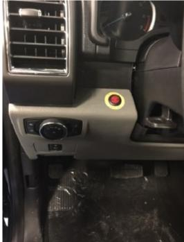
Route the orange and red harnesses across the dash to the streetside. Retain the harnesses under the dash, so that they do not interfere with the foot pedals and do not hang down in the foot area of the driver or passenger.
