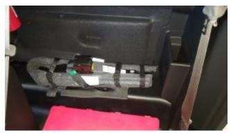
Reinstall jack by placing on mounting bracket studs and slide towards the driver side,
