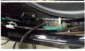
Remove the stepwell trim from the driver's door area. Pull the OEM ductwork out the way. Drill a 1/2" hole in the stepwell area. Apply self-etching primer to the hole. Insert the 3/8" ID grommet into the hole. Route the harness through the grommet and forward to the driver's kick panel area.
