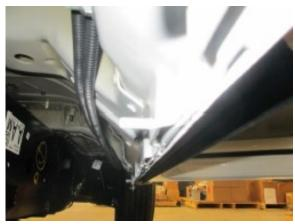
Underhood route the long red cable from the rear of the fuse holder and the long black cable rearward along the curbside to the bulkhead
