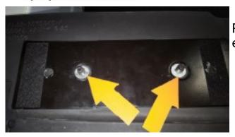
Put an FAS0317 nut on the bottom of each of the OEM studs and tighten
