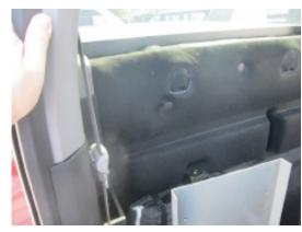
Assemble the 52930-G bracket to the bottom of the 52929-G plate with (3) FAS0018 screws and (3) FAS0055 nuts. The bottom of the plate has the hole in the center between two slots. Use the assembled inverter mounting plate as template to mark the locations for the fasteners to be drilled behind the rear passenger seat and the jack step.
