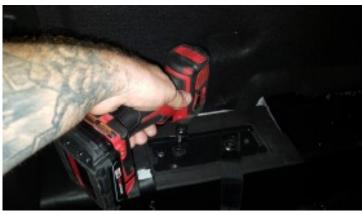
Remove the OEM jack mounting plate with T40 star bit.
