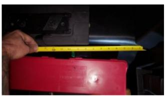
Place the modified OEM jack mounting bracket on step behind driver's seat. Measure 7.5" over from plastic B-Pillar trim.
