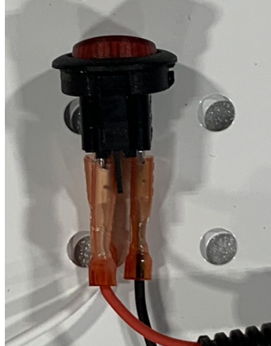
Diagram 7A-3: KIT 66008 & 66006 Remote Switch Connections
