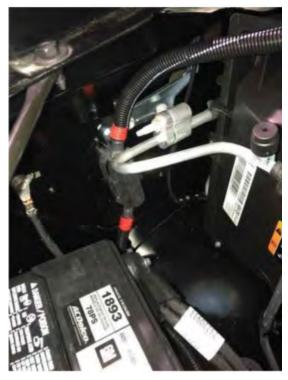
Mount the fuse holder to the inner fender with (2) FAS0682
