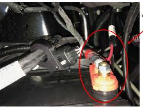
Remove the battery post screw on Wire Tie Here the OEM battery cable.
