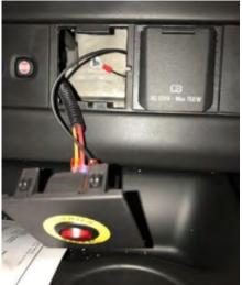
Ground the switch ground ring terminal to a metal structure with
