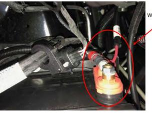
Remove the battery post screw on the OEM battery cable.
