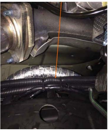
Keep the inverter wires away from the exhaust by routing along the frame, like seen in the picture.
