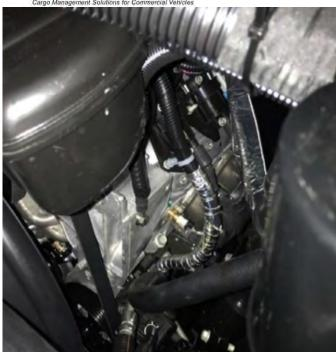
Connect the negative inverter battery cable to the hole in the block using (1) FAS0329, (1) FAS0588, and (1) FAS0552.
