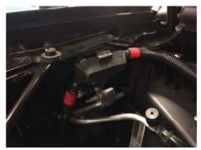
Mount the fuse holder to the inner fender with (2) FAS0682
