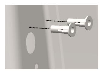
**Step 2:** Install the power strip and bracket to the D-pillar by using the 1/4" lock washers (FAS0060) and the 1/4-20x bolts (FAS0018)
