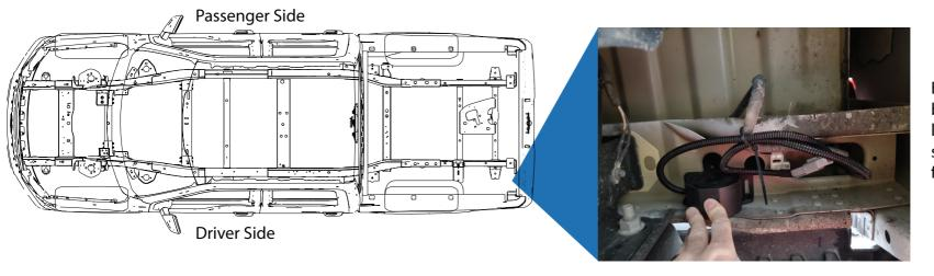
Backup alarm is located below the driver side tail lamp cavity on the street side of the driver side frame rail
