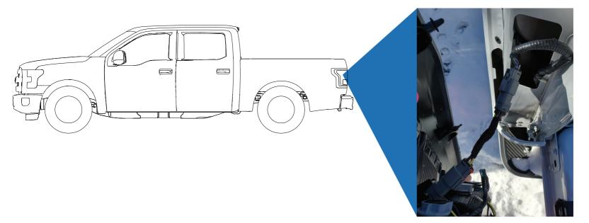
OEM tail lamp connector is located on back side of driver side tail lamp
