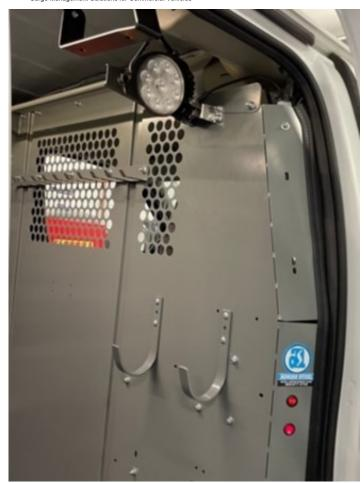
**Step 3:** Route the black and blue wire up the partition to the work light. Crimp the blue wire to the red wire of the work light, and then the black wires together.
