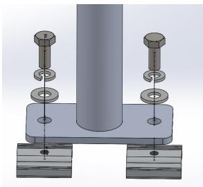
**Step 2:** Assemble the beacon mount feet by inserting the bolt (FAS0799) through the lock washer (FAS0588) then flat washer (FAS0552) then through the foot into the slide. Do not tighten down at this point.
