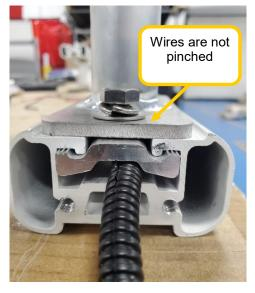
Step 4: There are two options for routing the wires. All wires will be routed through the roof into the cargo area on the driver side of the vehicle. All holes through the roof should be drilled as close to the rail foot as possible for wire routing.
