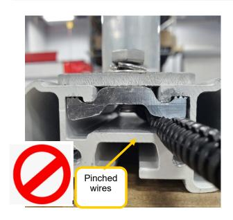
\*\*\*Be cautious the wires are not pinched after tightening the slides\*\*\*
