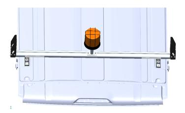
**Step 5:** Once the utility rack is mounted to the roof of the vehicle, drill a 47/64" hole in the roof, to the right of the foot mount. See the picture to the left for reference.
