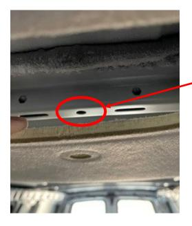
**Step 3:** Drill out the existing hole in the roof bow (where the trim retainer came out of) and insert the plusnut (FAS0052).
