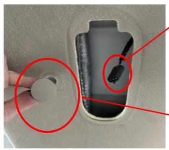
Cut the OEM connector off of the light. Make sure to leave plenty of length on the wires to attach to the new light.
