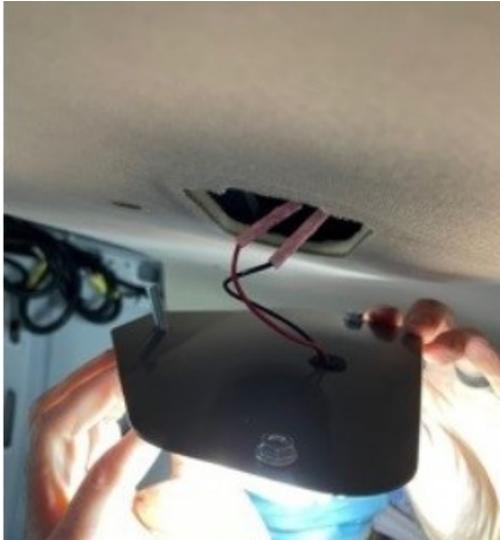
**Step 4:** Use the butt-connectors to attach the red wire from the light to the blue (positive) OEM wire, and the black wires together.
