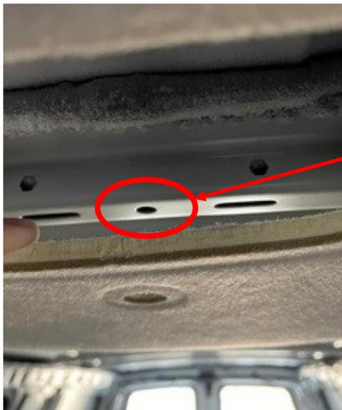
**Step 3:** Drill out the existing hole in the roof bow (where the trim retainer came out of) and insert the plusnut (FAS0052).
