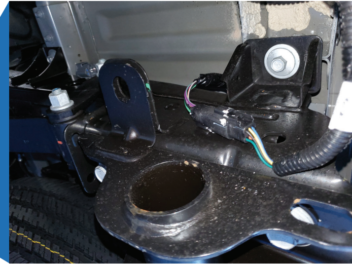
Inline connector is located on outside of driver side frame rail near rear of vehicle
