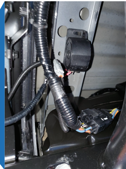
Backup alarm is located inside of driver side frame rail
