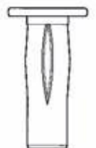
1/4" PLUSNUT P/N FAS0052 (INSTALLATION) "WINDSTAR ONLY"
