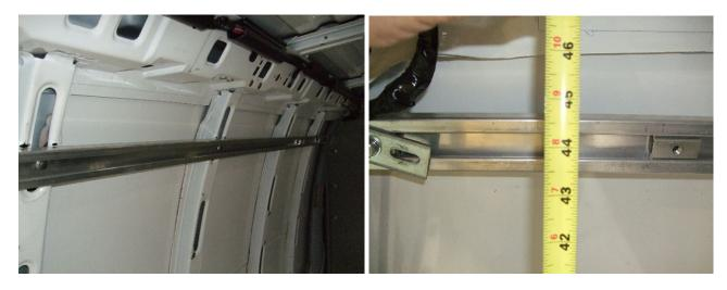
5. Insert (5) slides into rail. Install mounting bracket in upper rear corner, using (1) slide to fasten the bracket to the upper rail as shown below. Secure O.E.M. harness to the bracket with a wire tie at the wire holder.
