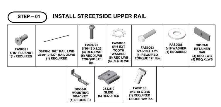
1. Locate hex hole in rear upper rear corner by removing wire holder. Drill and set plusnut.
