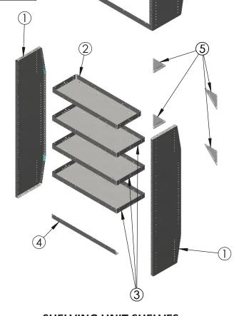
**SHELVING UNIT SHELVES** SF21244H-G, SF21444H-G, **AND GUSSETS GS6X6 ARE INSTALLED USING BAG00026-0**
