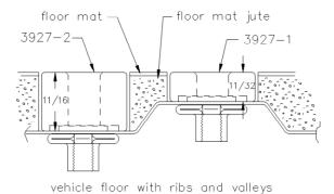
A PLUSNUT (RIVNUT) SETTING TOOL IS REQUIRED FOR PLUSNUT (RIVNUT) INSTALLATION AND IS SUPPLIED WITH THIS KIT. OR USE AN AIR POWERED PLUSNUT SETTING GUN.
