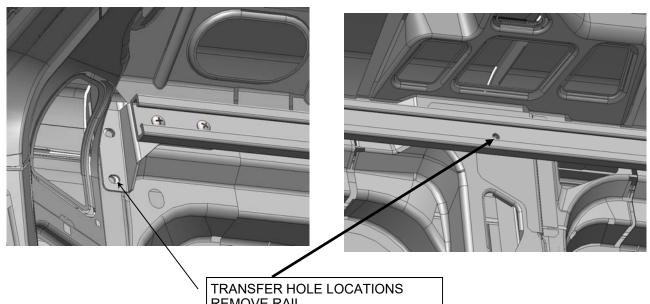
TRANSFER HOLE LOCATIONS REMOVE RAIL DRILL AND SET PLUSNUTS FAS0091—5/16 PLUSNUT (3)
