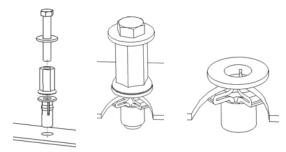
Place barrel of the plusnut body in sheet metal thru hole until flange is flush with sheet metal.
