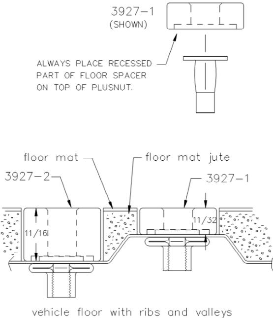
A PLUSNUT (RIVNUT) SETTING TOOL IS REQUIRED FOR PLUSNUT (RIVNUT) INSTALLATION AND IS SUPPLIED WITH THIS KIT. OR USE AN AIR POWERED PLUSNUT SETTING GUN.
