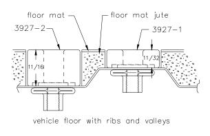
The location of various floor mounts will determine what spacer combination will be used. For example, an 11/32" spacer is used atop floor ribs, and an 11/16" high spacer is used atop floor valleys.
