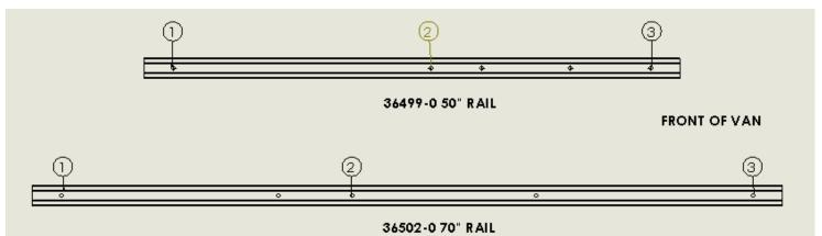
3. Slide rail so that it contacts wheel well as shown below. Measure 3.13" from the back end of the rail to the plastic trim, measure in the rear 11.25" to wall from outside edge of rail, front of rail 8.25" to wall from outside of rail as shown.
