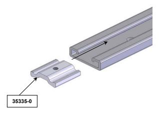
4. Install Front and rear brackets as shown below. The front bracket is attached to the rail with nut and bolt. The rear bracket is installed the same as the streetside. Secure O.E.M. harness to the bracket with a wire tie at the wire holder.
