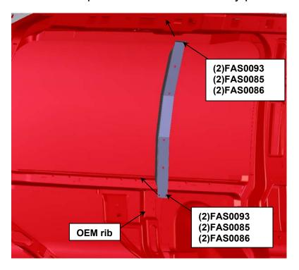
3. Install Front and rear brackets with rail as shown below. The front bracket is attached to the rail with nut and bolt. The rear bracket is installed the same as the streetside.
