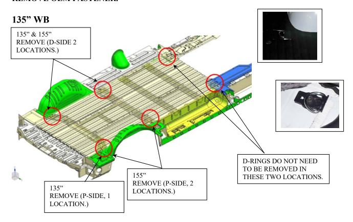
2. RE-INSTALL FASTENER – STOW D-RINGS FOR END USER, OR AS SPECIFIED PER PDS.
