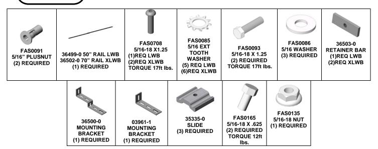
1. Locate hex hole in rear upper rear corner by removing wire holder. Drill and set plusnut. On rear side of the C-pillar measure up 44" from the top of the floor rail mark and drill for plusnut. Install plusnut as shown below
