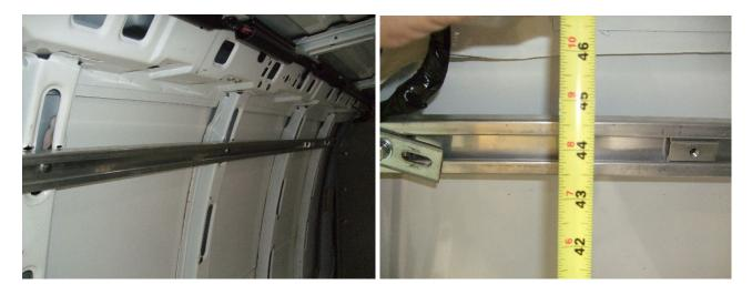
5. Insert (5) slides into rail. Install mounting bracket in upper rear corner, using (1) slide to fasten the bracket to the upper rail as shown below. Secure O.E.M. harness to the bracket with a wire tie at the wire holder.
