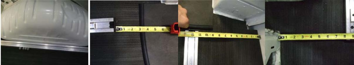
**NOTE: VERIFY DISTANCE BETWEEN FLOOR RAILS IS 48" MINIMUM, OVER 48" IS ACCEPTABLE.**
