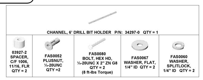
Reposition the Channel as shown below and secure to the vehicle bed rail using the fasteners listed below. Install all (3) set of fasteners prior to final tightening to final torque specifications.
