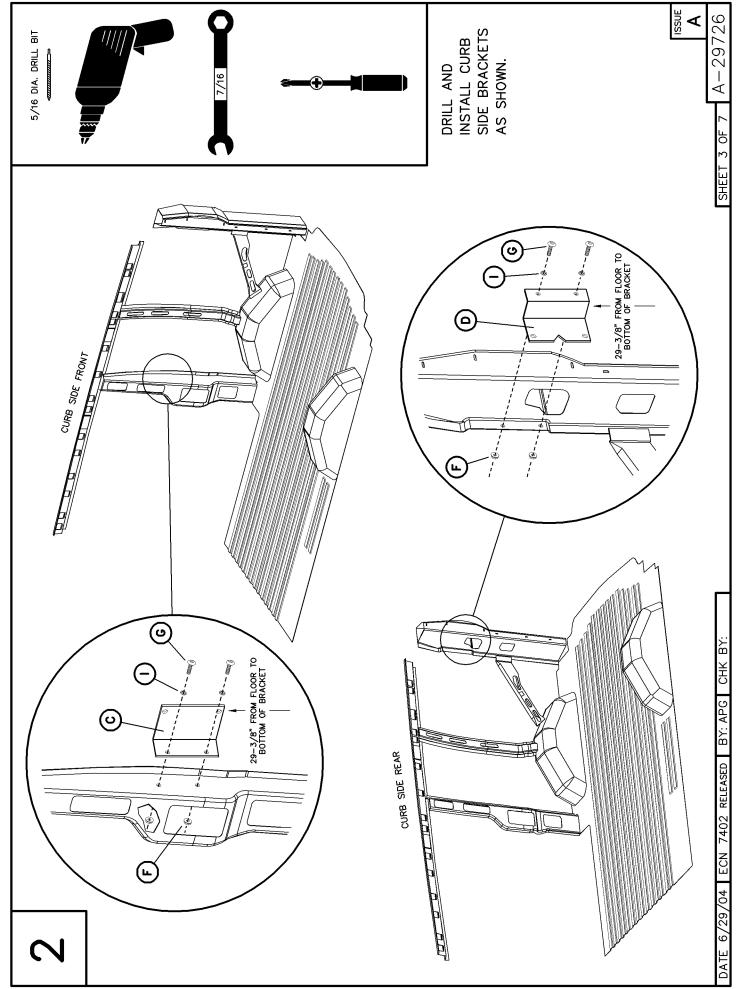
IF A VAN LINER IS USED WITH THIS E—TRAC KIT, THE LINER SHOULD BE INSTALLED AFTER THE PLUSNUTS ARE PLACED IN THE BRACKETS, AND BEFORE THE E—TRAC IS INSTALLED.
