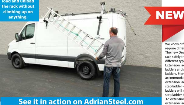
We know different jobs require different ladders. The new Drop-Down ladder rack safely transports all different types of ladders. Extension ladders, step ladders and specialty ladders. Standard rack accommodates 28' extension ladder and 10' step ladder – short step ladders will need optional step ladder kit and up to 32' extension ladder with extension ladder kit.
