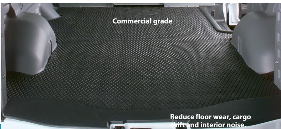
**Floor Mats** are die-cut for wheelwells and meet flammability test MVSS 302. Made of 3/16" rubber, diamond corrugated pattern. Side stepwell and seat pedestals require some trimming.
