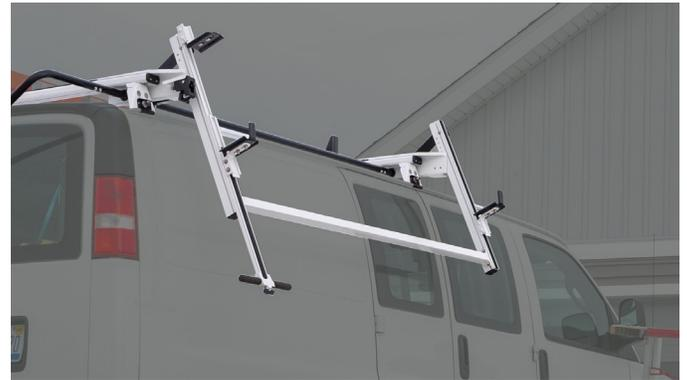
**Max-Drop ProLift™** has a single function that lowers the ladder to a single set height and a secondary function that lowers the rear of the ladder even further to a safer more ergonomic height. Most similar to our previous DDLR drop down series.
