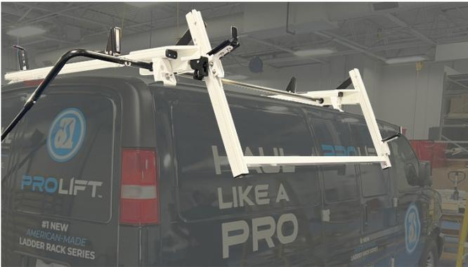
**Standard-Drop ProLift™** has a single function that lowers the ladder to a single set height. Uses hook brackets to hold and secure ladders.
