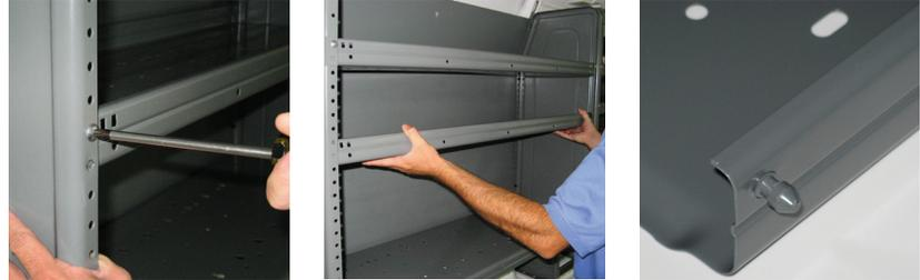
**Truly Adjustable Shelves** All you need is a phillips screwdriver! Simply remove two bolts from the speed nut clips that come with the shelf, tilt the shelf upwards, move the shelf to your desired location, insert the rear shelf studs, reattach the bolts and you're done!
