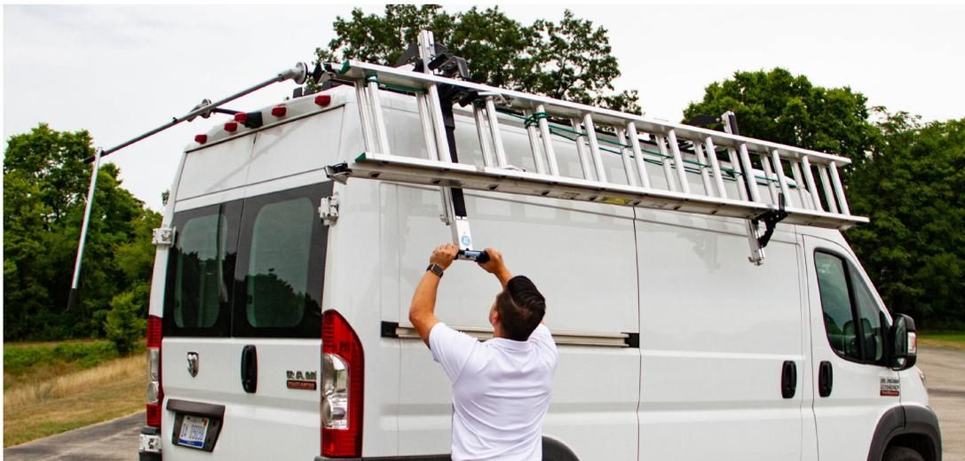
Standard rack accommodates 28' extension ladder and 10' step ladder – short step ladders will need optional step ladder kit and up to 32' extension ladder with extension ladder kit.
