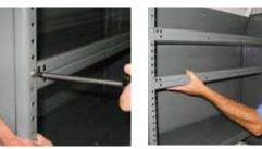
Truly Adjustable Shelves All you need is a phillips screwdriver! Simply remove two bolts from the speed nut clips that come with the shelf, tilt the shelf upwards, move the shelf to your desired location, insert the rear shelf studs, reattach the bolts and you're done!
