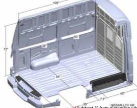
Subtract 3" from dimension when a Max Comfort partition wing kit is installed.
