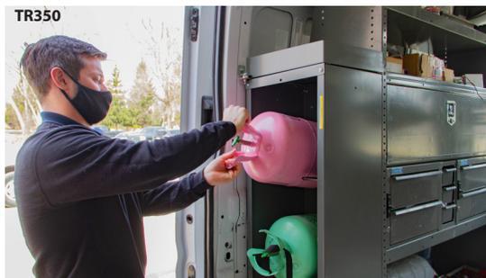
Safely carry 30-lb. and 50-lb. refrigerant tanks securely in your van. Tank Racks can be installed for easy access from the side or rear van doors for increased ergonomics and reduced risk of injury. For customers with a high roof van, these products can be stacked to carry more tanks by using the vertical space in you van.
