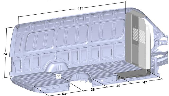
**Sprinter High Roof 170" Extended WB 2007-newer**
