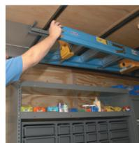
**1** Simply press ladder inward to release rear ladder rung from the rear damp bracket.
