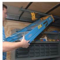
**3** Remove front rung from the front clamp bracket and you're ready to go to the job site!
