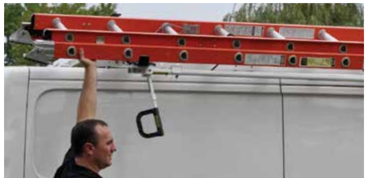
Lift ladder off the rear bracket.
