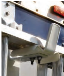
Plastisol ladder clamps protect fiberglass ladders
